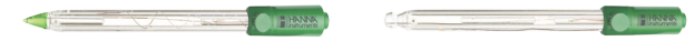
HI10530 Triple ceramic, double junction, glass body, refillable pH electrode with conical tip and temperature sensor Recommended for fats, creams, soil and low conductivity samples
