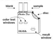
Add to the other vial deionized water up to the 10 mL mark. Replace the cap and shake to mix.
