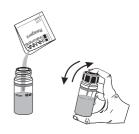
Add one packet of HI93709B-0 Manganese High Range Reagent B. Replace the plastic stopper and the cap. Shake gently for 2 minutes to mix.
