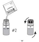
Add 0.5 mL of HI96773B-0 Oxygen Scavengers Reagent B to each cuvette using the 1 mL syringe.
