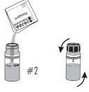
Add 0.5 mL of HI96773B-0 Oxygen Scavengers Reagent B to each cuvette using the 1 mL syringe.
