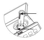
5. Using light pressure, push the adapter down until it reaches the bottom of the meter's cuvette holder. When the vial adapter reaches the bottom, you should no longer be able to see the notched area of the adapter.
