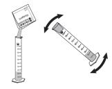
Add one packet of H193730B-0 Molybdenum Reagent B to the cylinder, close and invert several times until completely dissolved.
