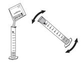
Add one packet of HI93730C-0 Molybdenum Reagent C to the cylinder, close and shake vigorously.
