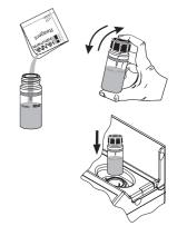
• Press **Timer** and the display will show the countdown prior to the measurement or wait 3 minutes and press Read 2. The instrument displays the result in mg/L of Iron(III) (Fe<sup>3+</sup>).
