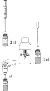
Replace the plastic stopper and the cap. Invert several times to mix.
