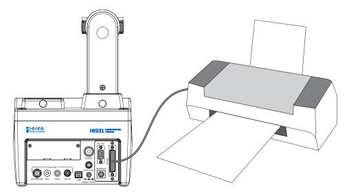
Warning: The titrator and the external printer must be both turned off before they are connected.
