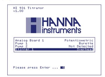
**Note:** All the performed initialization processes must be successfully completed. If one fails, restart the titrator. If the problem persists, contact your nearest Hanna Instruments Service Center.
