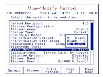
If one of the options (V-Blank or Blank-V) is selected in the **View / Modify Method** screen, the *blank value* will be active on the **View / Modify Method** screen and the value of the blank can be set (in liters).
