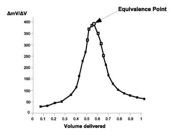
The detection algorithm looks for the maximum value of the 1<sup>st</sup> derivative. The 1<sup>st</sup> derivative must be greater than the threshold value at the maximum point. See **4.5.7**. **RECOGNITION OPTIONS (EQUIVALENCE ENDPOINT ONLY)** section for more information.
