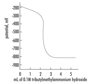
Figure 7: Non-aqueous titration
