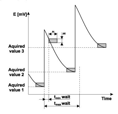
The signal stability window (condition) represents the time interval ( $\Delta t$ ) during which the potential measured in solution (mV) is confined inside the potential interval ( $\Delta E$ ).
