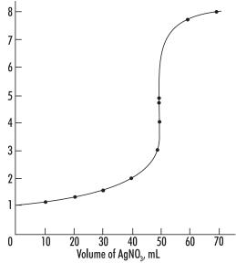
Figure 5: Argentometric titration
