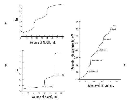
Figure 9: Multiple endpoint titrations
