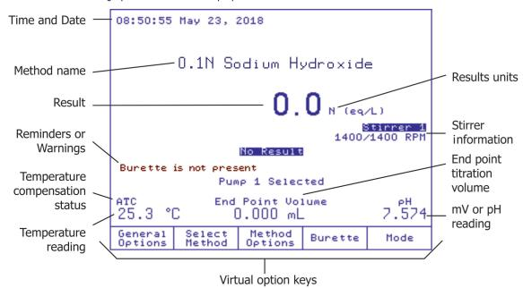
The titrator has a 5.7" graphical backlit color display.
