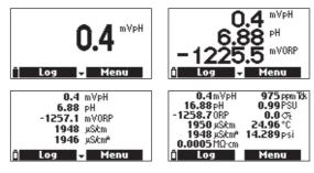
A blinking measurement value indicates that the measurement is out of range.
