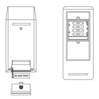
• HI 93501, HI 93502, HI 93503 and HI 935007: the batteries are accessed by separating the front and the back halves of the meter. Unscrew the 4 screws on the back of the meter and carefully replace the three 1.5V AA alkaline batteries located in the battery compartment, while paying attention to their polarity. Reattach the back making sure that the gasket is in place and tighten the 4 screws to ensure a watertight seal.
